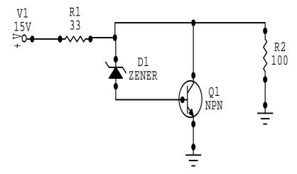
2. Calculate the regulated output voltage in the ckt of fig.
